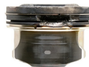
Piston head after 10,000 miles Damage from LSPI
